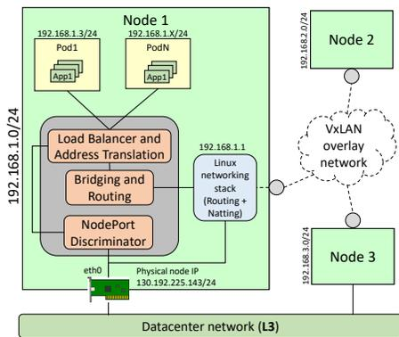
Fig. 2: Architecture of the Polycube K8s plugin.
